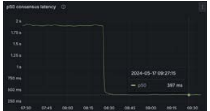
Fig. 1: P50 latency of a major blockchain switching from Bullshark (1900ms) to MYSTICETI-C (390ms) consensus on 106 independently run validators
